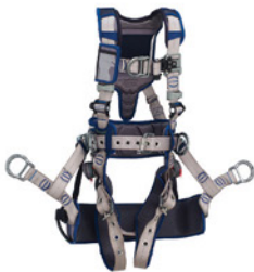
ExoFit STRATA Tower Climbing Harness Tongue buckle leg straps, aluminum front, back and side D-rings, removable seat sling with positioning D-rings.
